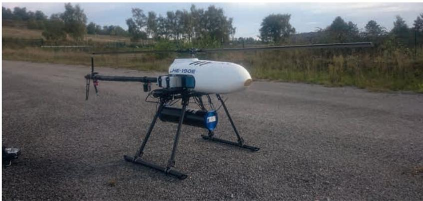
**Figure 6** The petrol-powered drone used for mapping the mine tailing. Underneath the 1 litre MS-1000 gamma-ray sensor.
