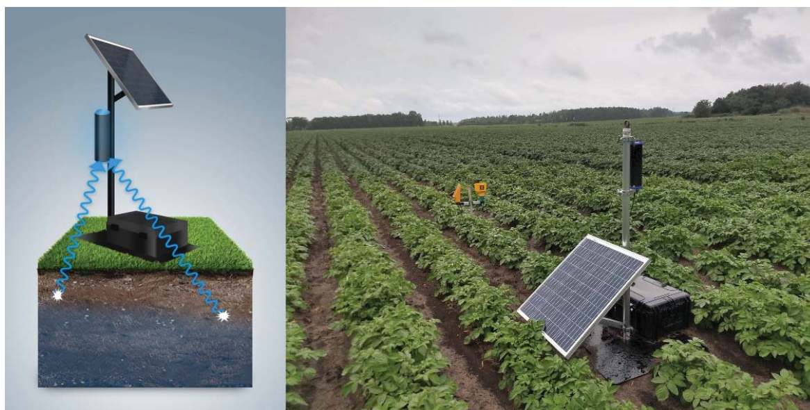
Fig. 6.8. Left: schematic drawing and picture of the gSMS sensor setup in the field. The black tube with blue caps mounted on a pole represents the gamma-ray sensor. The box on the ground is a schematic representation of the battery continuously recharged by the solar panel. In practice, this battery container is small compared to the measurement footprint so that it does not block a significant portion of the gamma-rays emitted from the soil. The blue wiggles in the schematic drawing represent the gamma radiation from the soil, measured by the sensor. Right: a picture of the setup in an agricultural field that is used to grow potatoes.
