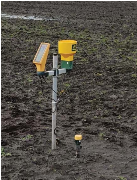
Fig. 6.9. Dacom TerraSen pro sensor. The probe on the bottom of the picture is inserted into the soil and contains the moisture sensors at five depths. The yellow cup on the top right of the stick is the rain gauge, and the solar panel on the top right is used to charge the sensors' internal battery.
