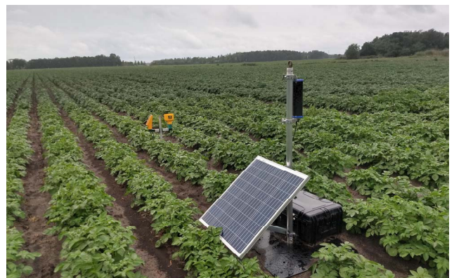
Fig. 3: Medusa and Dacom sensors placed in a potato field in the north-east of the Netherlands. The black tube with the blue caps is the gSMS and the yellow sensors in the background are the Dacom TerraSen moisture sensors.
