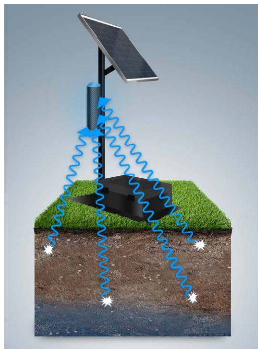
Fig. 1: Schematic representation of the gamma Soil Moisture Sensor. The sensor measures gamma-radiation emitted by the soil under the sensor. If the moisture in the ground increases the amount of radiation is attenuated.
