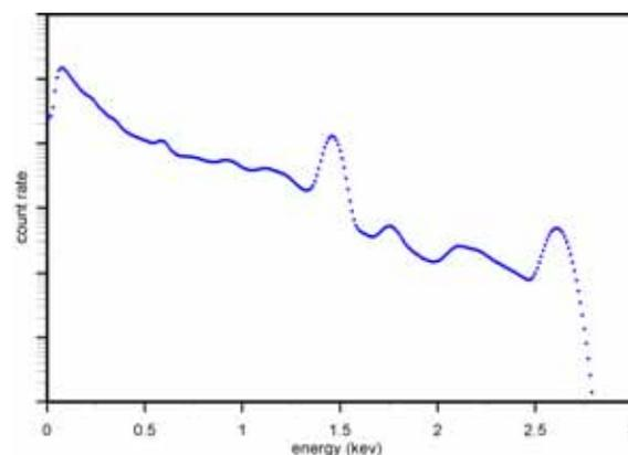
Figure 1. Sample spectrum of natural gamma radiation. The peak structure contains information on the contributing radionuclides.
