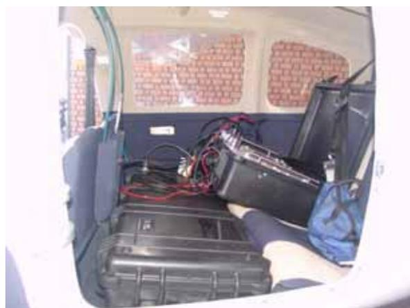
Figure 6. Detector (lower box) and readout system (upper box) in the back of the plane.
