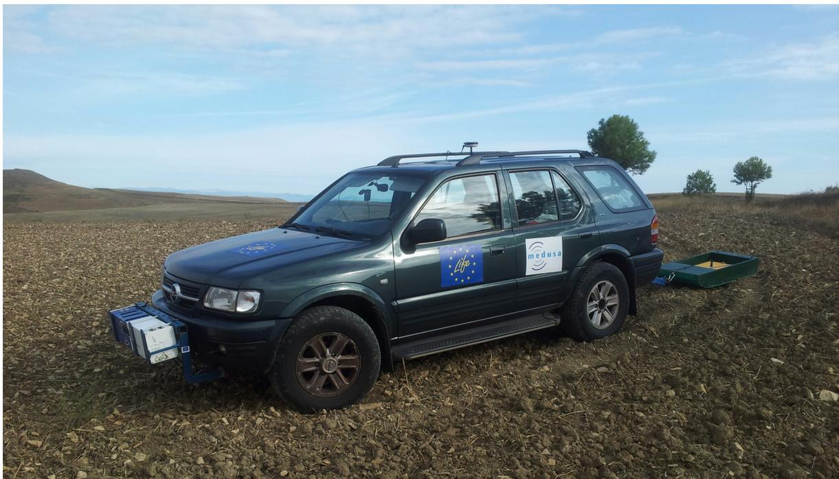
**Figure 2** Measurement setup with a gamma-ray spectrometer in front of the vehicle and GPR behind in a carriage the vehicle.
