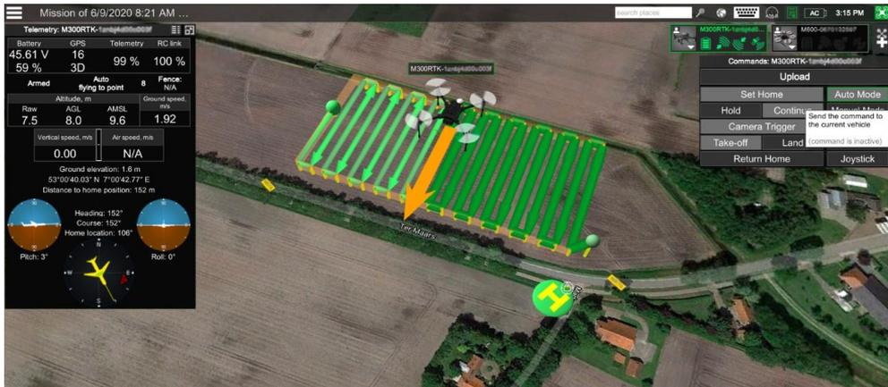
**Fig. 1.4.** A typical view of the software used to prepare and execute a UAV survey. This screenshot shows the software package UgCS, version 4.6.520 (UgCS, 2022). An evenly spaced grid is used in this UAV survey. Flight planned, executed and screenshot generated by vliegend.nl (Vliegend.nl, 2022).
