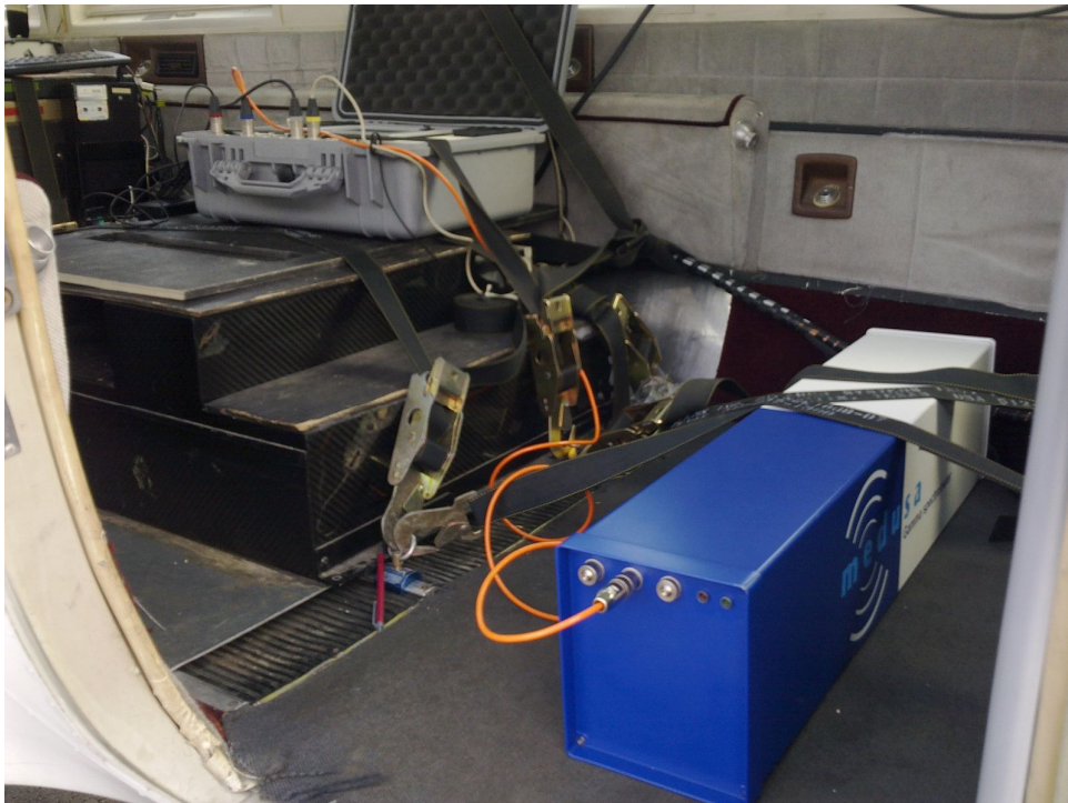
Figure 2: Medusa system (right) mounted next to one of the 16L systems (black box on the left)
