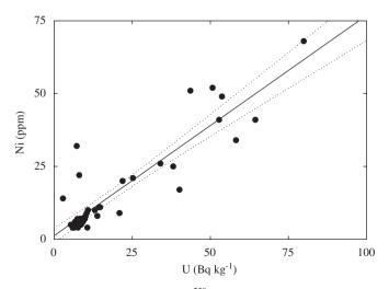
Fig. 1. Correlation between Ni and  $^{238}$ U in Meuse and Rhine sediments. Solid line is linear regression Ni (ppm) = 1.26 + 0.76U (Bq kg<sup>-1</sup>) ( $R^2 = 0.82$ ). Dotted lines are 95% confidence intervals.
