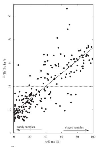
Fig. 7.  $^{232}$ Th activity concentration (Bq kg<sup>-1</sup>) as a function of the fraction of grain sizes  $<63 \,\mu\text{m}$ . The dotted line represents the Th = 20 Bq kg<sup>-1</sup> level at which the total data set has been split. The solid line is a least-squares fit to the total data set.
