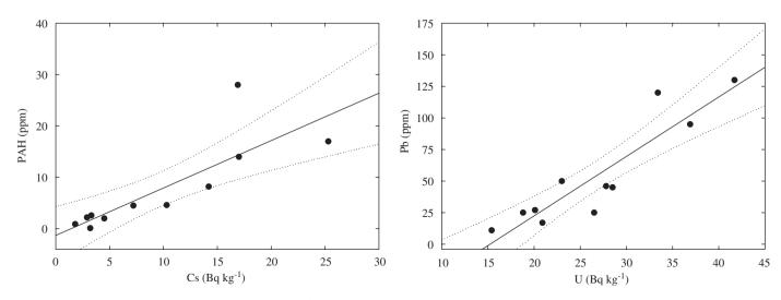
Fig. 9. Correlation plots from a project in the harbour of Deventer, the Netherlands. Solid lines are linear regressions: PAH (ppm) =  $-1.3 \pm 0.9$  Cs (Bq kg<sup>-1</sup>) ( $R^2 = 0.70$ ) and Pb (ppm) =  $-71.6 \pm 4.71$  U (Bq kg<sup>-1</sup>) ( $R^2 = 0.83$ ). Dotted lines are 95% confidence intervals.
