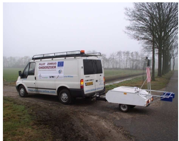
Figure 2: Example of fieldwork with the gamma spectrometer placed in a small car behind the van.
