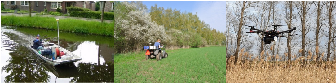
Figure 3: a gamma-ray spectrometer can be towed behind a vessel for mapping aquatic sediments, can be mounted on a quad bike for mapping accessible floodplains and can be connected to a drone for mapping terrain that is difficult to access.
