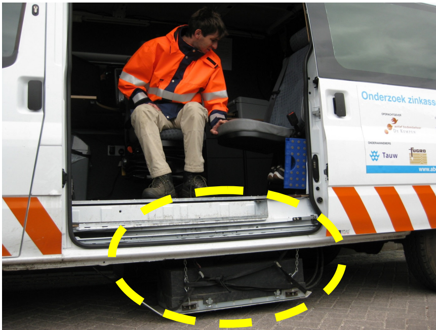
Figure 7: the GPR (black box under the car) is mounted under the vehicle.
