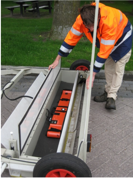
Figure 5: the EM sensor is mounted behind the vehicle in a non-conductive carriage.
