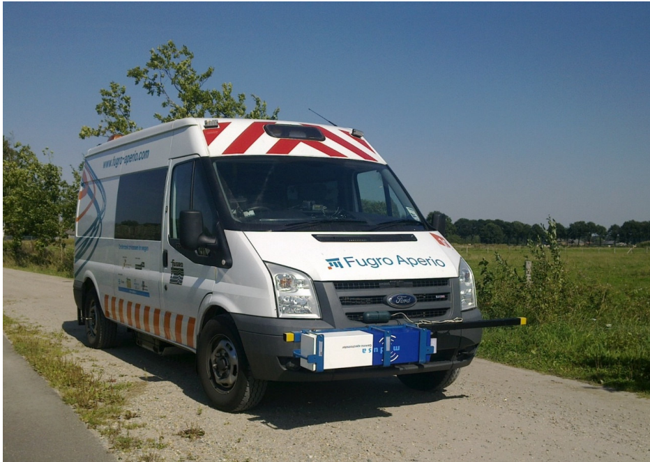
Figure 3: Spectral gamma sensor mounted on the front of the measurement vehicle.
