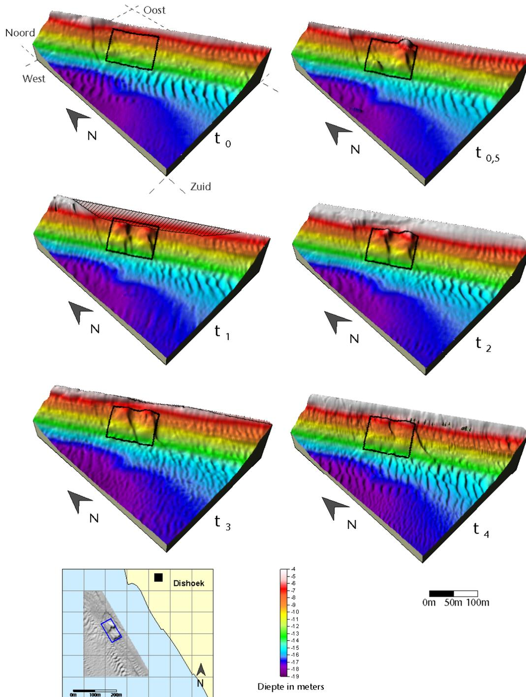
Fig. 4. 3D image of the bathymetry of the nourished site, during six surveys. The rectangle represents the predetermined dump site.  $t_0$  = September 18, 2001;  $t_{0,5}$  = October 24, 2001;  $t_1$  = November 10, 2001;  $t_2$  = December 3, 2001;  $t_3$  = February 18, 2002;  $t_4$  = October 7, 2002
