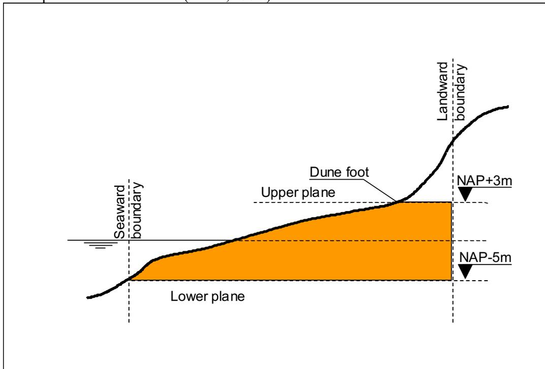
Fig. 1. Cross sectional area used to determine the position of the Momentary Coastline (MCL)
