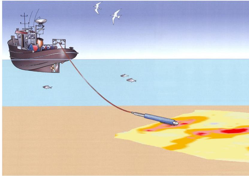
Fig. 3. The MEDUSA system towed behind a vessel
