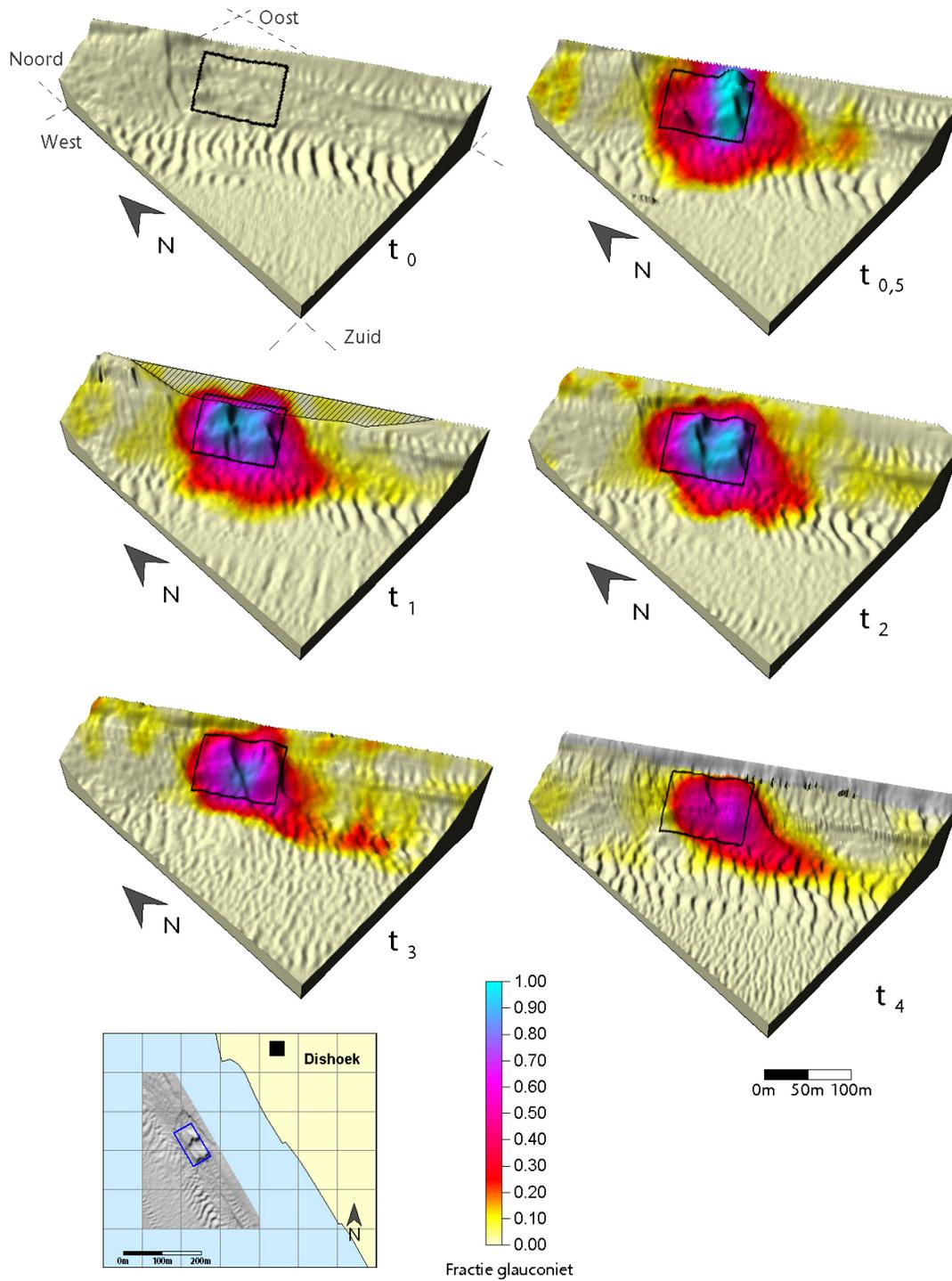
Fig. 5. Distribution (in color) of the fraction of glauconitic sand, projected on the 3D bathymetry images.  $t_0$  = September 18, 2001;  $t_{0,5}$  = October 24, 2001;  $t_1$  = November 10, 2001;  $t_2$  = December 3, 2001;  $t_3$  = February 18, 2002;  $t_4$  = October 7, 2002
