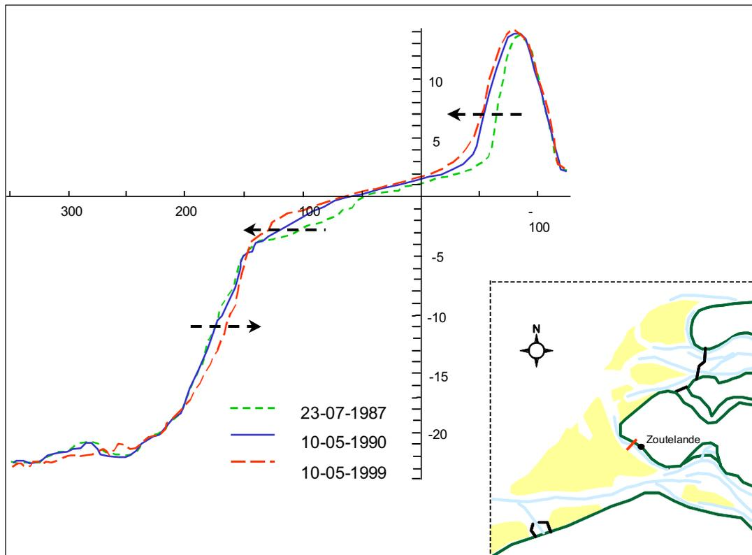
Fig. 2. Typical profile of the Oostgat and development of the profile over a 12 year period
