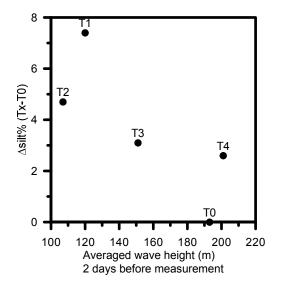
*Figure 7: Change in average silt content as function of averaged wave height before the measurement.*
