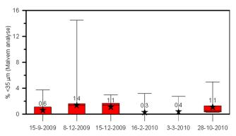
Figure 3: Box-whisker plot of the % <35  $\mu$ m of sediment samples of different campaigns, measured with the Malvern particle sizer. A star (with number) shows the average.
