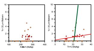
Figure 4: scatterplot of silt content (%<35 $\mu$ m, measured on a Malvern) vs potassium and U+Th for sediment samples taken during the project. The red line present a linear fit of the samples with a silt content >0.3% and <3%. The green line presents the fingerprint of SPM (see Figure 2).
