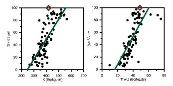
Figure 2: scatterplots of silt content (%<63 $\mu$ m) vs potassium and U+Th for sedimentsamples from various projects around the North Sea..The resulting numbers of clay fraction are derived from different systems (Malvern, sieving).The brown datapoint is based on measurements of SPM. Only datapoints with a silt fraction >3% are plotted.
