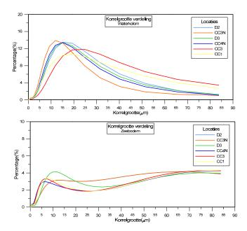
Figure 1: Sieve analysis of sediment in suspension (upper figure) and seafloor sediments. Prior to analysing, the grains >90  $\mu$ m were removed by sieving
