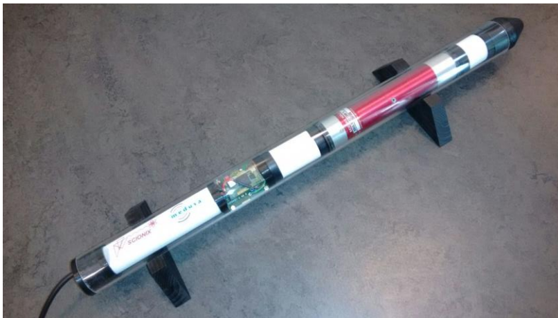
Figure 1. Test setup of a 1x1 inch CeBr tool coupled to the 1024 channel readout system. The diameter of the system shown is around 30mm.
