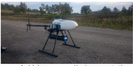
**Figure 6** The petrol-powered drone used for mapping the mine tailing. Underneath the 1 litre MS-1000 gamma-ray sensor.
