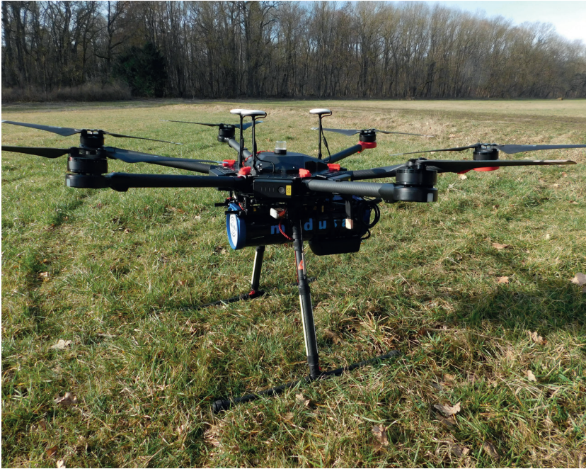
▲ Figure 4: MS-1000 gamma-ray spectrometer mounted under a standard commercial DJI M600 drone.
