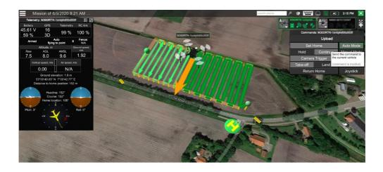
**Fig. 1.4.** A typical view of the software used to prepare and execute a UAV survey. This screenshot shows the software package UgCS, version 4.6.520 (UgCS, 2022). An evenly spaced grid is used in this UAV survey. Flight planned, executed and screenshot generated by vliegend.nl (Vliegend.nl, 2022).
