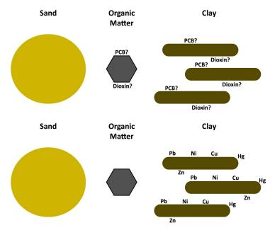
Figure 5: Top: organic pollutants that are diffusely distributed in the water column will mainly bind to clay particles and organic matter complexes (Uddin, 2017). Bottom: heavy metals mainly adsorb to clay particles (lower image). Scientific laboratory analyses are described in (van der Graaf et al., 2007). A review (Uddin, 2017) describes how "adsorption is one of the most important processes of metal uptake by clay".
