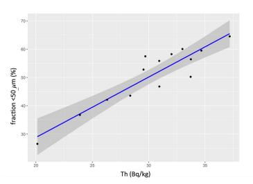
Figure 6: the application model that translates the thorium concentration (Bq/kg) into the clay fraction, defined as the grain size <50µm.
