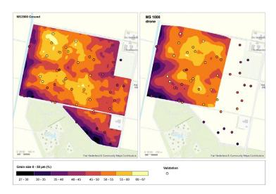
Figure 7: grain size map derived from a ground-borne survey (left) and an droneborne survey (right).
