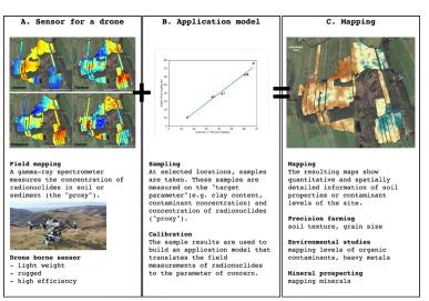
Figure 1: the 3-step approach for sensor-based mapping, the application model to a map that can be used by an end-user.
