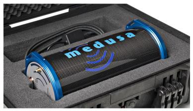
Figure 3. The MS-1000 Drone Detector is a low-power and robust gamma-ray detector system and, with a weight of 6.3 kg, is intended for use under UAV's.
