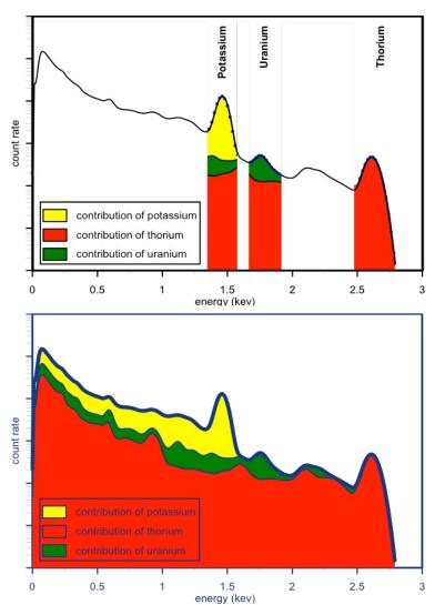
Figure 2. In the windows approach of data analysis, only part of the measured data is used (top). In the FSA approach (bottom), all data is used and every last piece of information is squeezed out of the spectral data.
