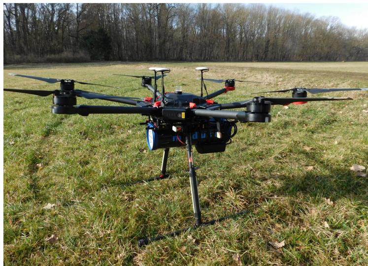
Figure 8: MS-1000 gamma spectrometer mounted under a standard commercial DJI M600 drone.
