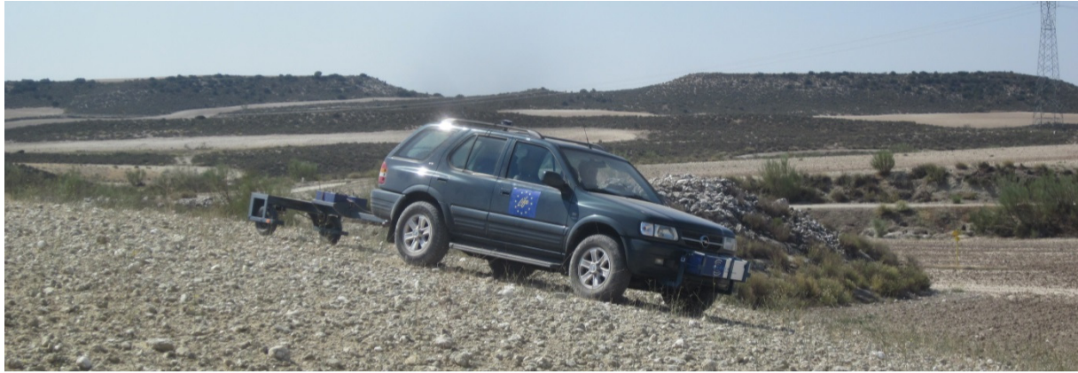
Figure 2. Measurement setup with a gamma spectrometer in front of the vehicle and GPR behind in a carriage the vehicle
